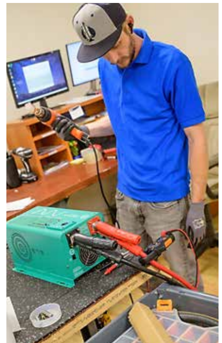
Jepsen fault checks an inverter that was returned earlier in the day.
